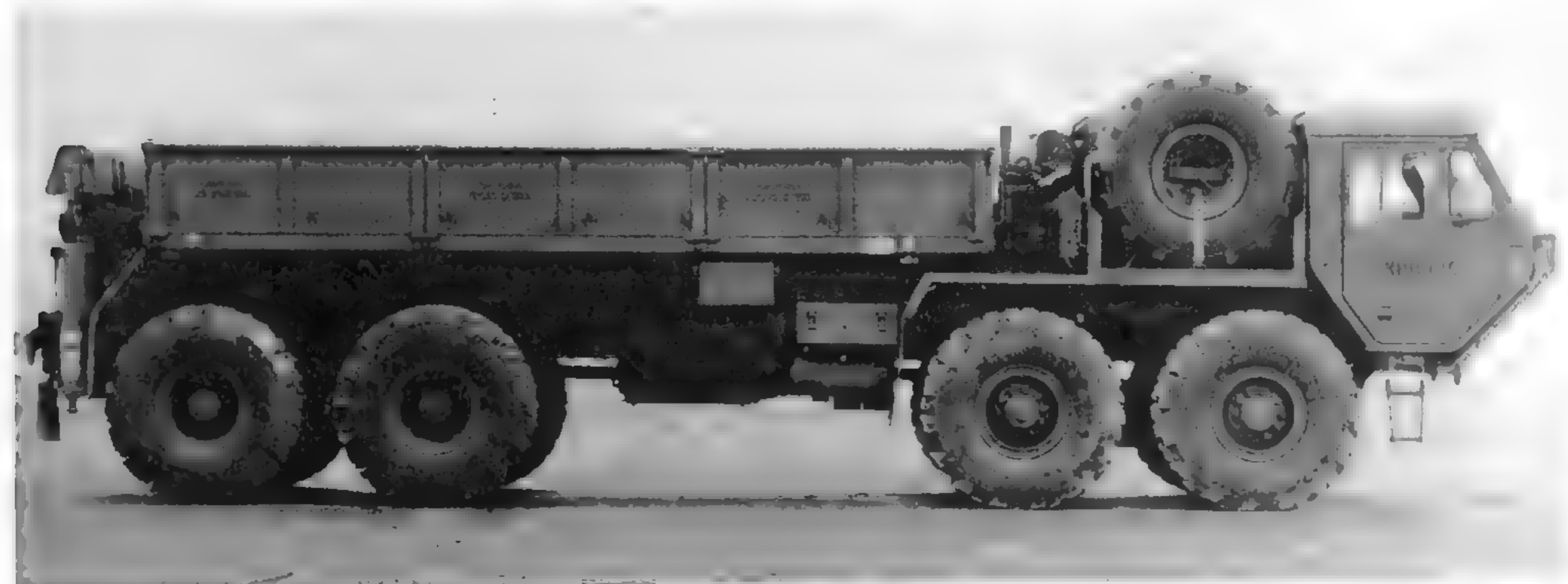
The angular cab-forward design of the Oshkosh M977 HEMTT makes it look like one of the airport crash trucks built by the same firm than a military vehicle. (U.S. Army photo)
